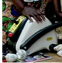
The WEZA machine is a generator that can be pumped by foot or hand
